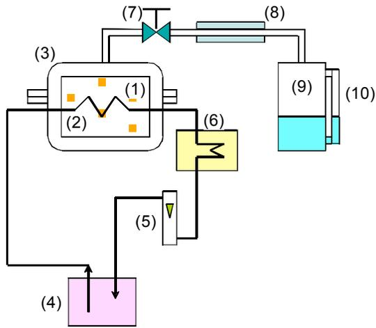
Figure 1: Laboratory-scale MgO/H<sub>2</sub>O chemical heat pump: (1) packed bed reactor, (2) heating tube, (3) reactor chamber, (4) thermostat, (5) flow meter, (6) radiator, (7) stop valve, (8) condenser, (9) water reservoir, (10) water level meter.
