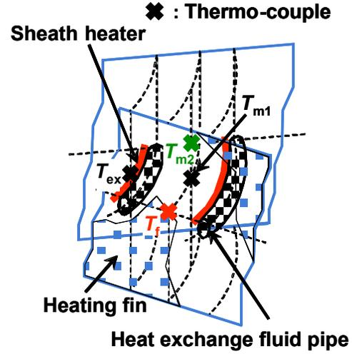
Figure 2: Cross section of reactor bed cut vertically to the radius direction
