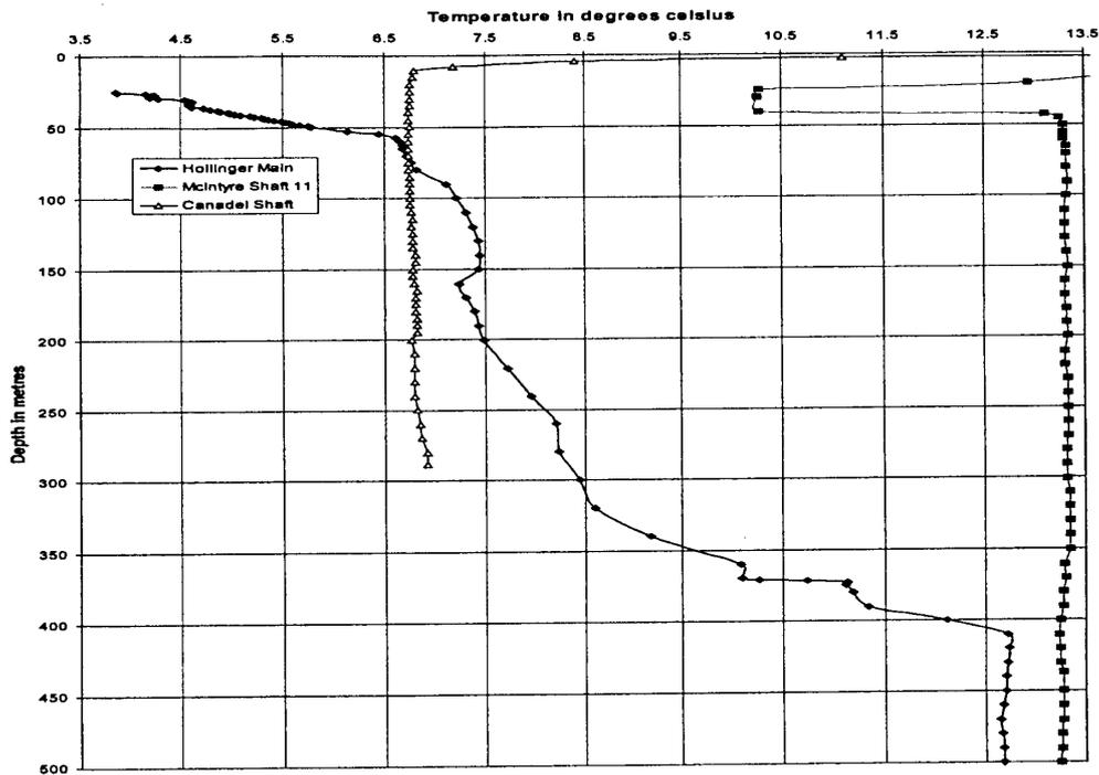
Figure 2: Temperature profiles for the Hollinger Main Shaft, McIntyre Shaft 11 and Canadel Shaft in Timmins, Ontario.
